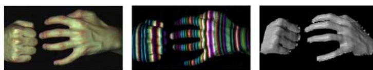
Figure 5.3.2: From left to right: two complex physical objects, a pattern of colored straight lines and their deformation when hitting the surfaces, reconstructed 3D shape. From (Zhang et al. 2002).
