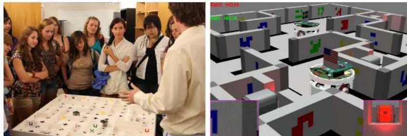
Figure 17.1.1: The “Ratslife” maze competition created from LEGO bricks and e-Puck robots (left). The same environment simulated in Webots.
