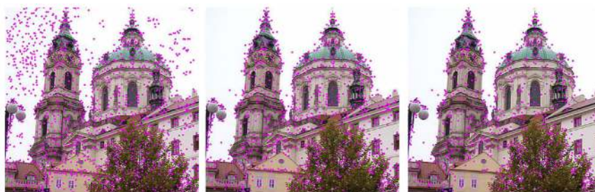
Figure 7.4.2: After scale space extrema are detected (left), the SIFT algorithm discards low contrast keypoints (center) and then filters out those located on edges (right). © Lukas Mach CC-BY 3.0
